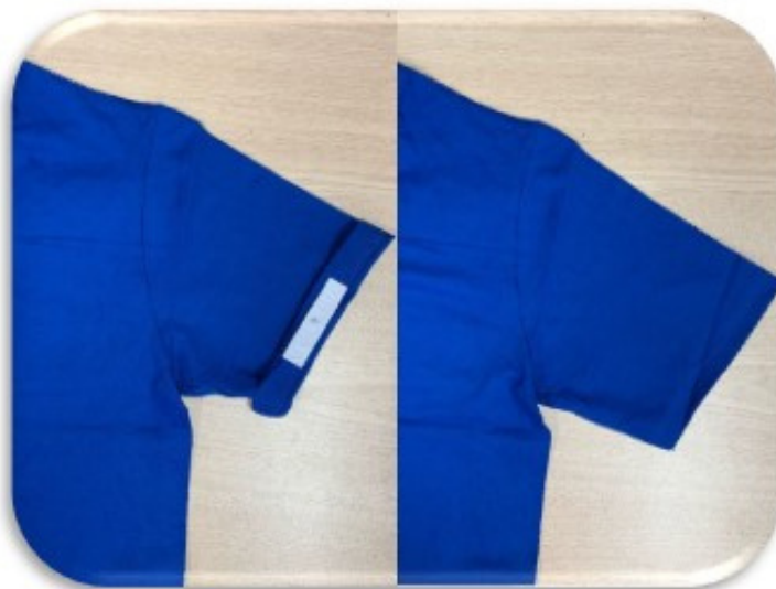
Small and water proof RFID tag/s sewn into the seams of residents' clothes
